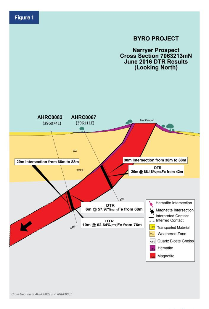
From within the intersections reported 29 July 2016, Table 1, a total of 99 samples were selected for Davis Tube Testing. The samples from each intersection were selected and combined to form composites representative of each intersection. A total of 31 composites were assembled and following a grind establishment were milled to 90µm to achieve liberation of the magnetite ore.
